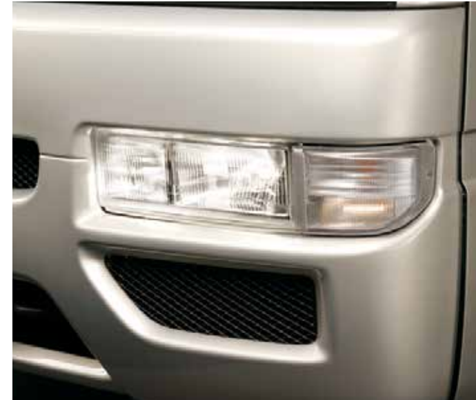
Halogen headlamps and fog lamps (GL) increases nighttime and inclement weather visibility.
