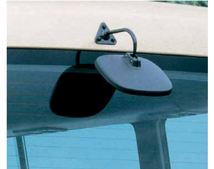
Rear-mounted outside mirror improves visibility when reversing.
